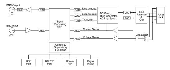
The DC output impedance is fixed at 200  $\Omega$  for each of the tip and ring leads, while the AC output impedance can be selected from 3 standard values (600  $\Omega$ , 900  $\Omega$ , TBR-21 Complex). An optional 4<sup>th</sup> impedance can be factory installed at the time of ordering.
