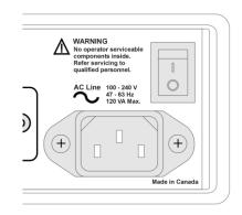
Connect the AC power cord, ensuring a snug fit to the receptacle. Turn on the power to the AI-7280 by rocking the power switch upward.
