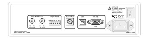
The two BNC connectors can either monitor various signals internal to the AI-7280 or inject signals into the AI-7280. The BNC input connector is AC coupled and withstands a maximum DC voltage of 55 volts. It can accept a maximum peak-to-peak signal of 5 volts with an AC input impedance of 100 k  $\Omega$ . The BNC output connector is DC coupled and outputs a maximum of 5 volts peak-to-peak with an output impedance of 600  $\Omega$ .
