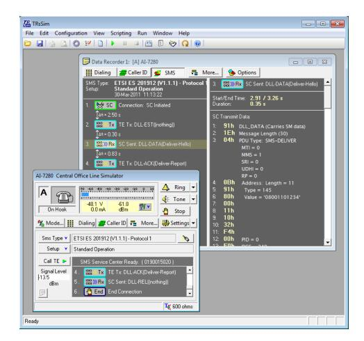
The SM-SC option supports both the ETSI ES 201 912 protocol 1 or protocol 2 standard. Designed as a testing tool, the software allows complete control over the DLL (data link layer) and TL (transfer layer) messages for exception condition testing.
